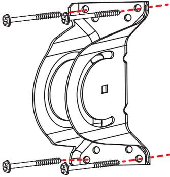
Find the four mounting screws included in this package. Using these screws, attach the base to the surface as shown here.
