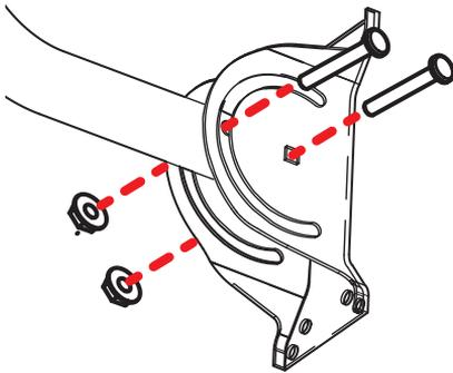
Insert the mast into the middle of the mounting base as illustrated here. Then insert one of the 1/4"x20 mounting bolts through the bottom hole on the side of the mounting base and mast as shown. Screw one of the hex nuts onto the end of the bolt to hold the mast and base together. Don't tighten the nut completely yet.
