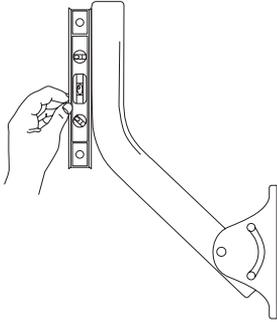
Position the mast so that it's perpendicular to the ground (plumb). Then tighten the two hex nuts to hold the mast in this position.
