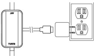
Plug the antenna's USB-powered amplifier into a USB power adapter (not included).
