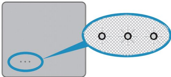
Move your antenna until the signal meter shows at least the second indicator. For best performance, try to get the third indicator.
