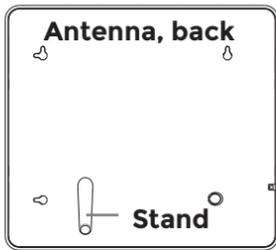
This antenna offers two placement options: the provided stand or wall mounting. If you'd like to use the stand, insert it into one of the circular slots on the back of the antenna. The antenna can be positioned vertically or horizontally.
