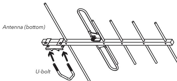
Screw the two wingnuts on the U-bolt so that the mounting bracket is held on the antenna.
