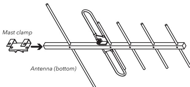
Place the U-bolt through the holes on both sides of the mast clamp.
